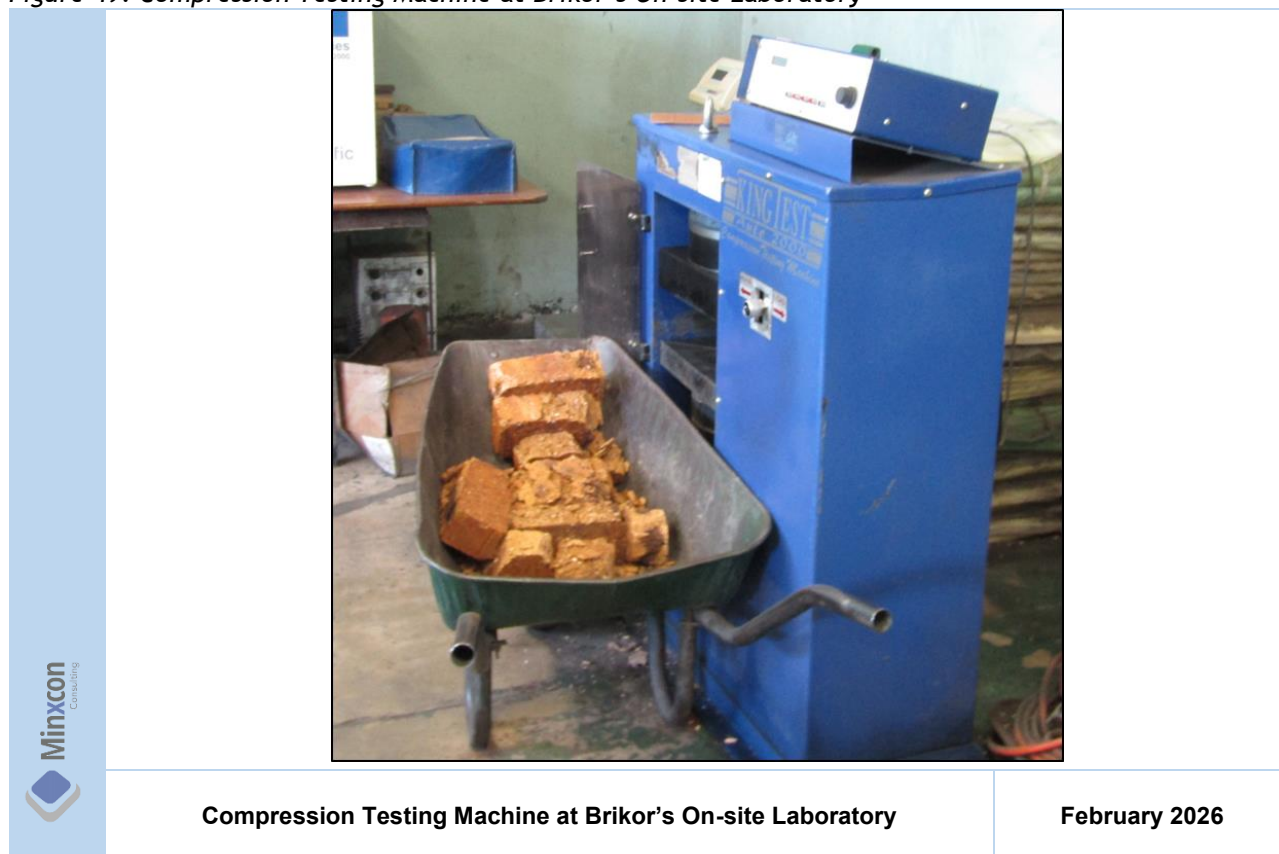
Figure 49: Compression Testing Machine at Brikor's On-site Laboratory
