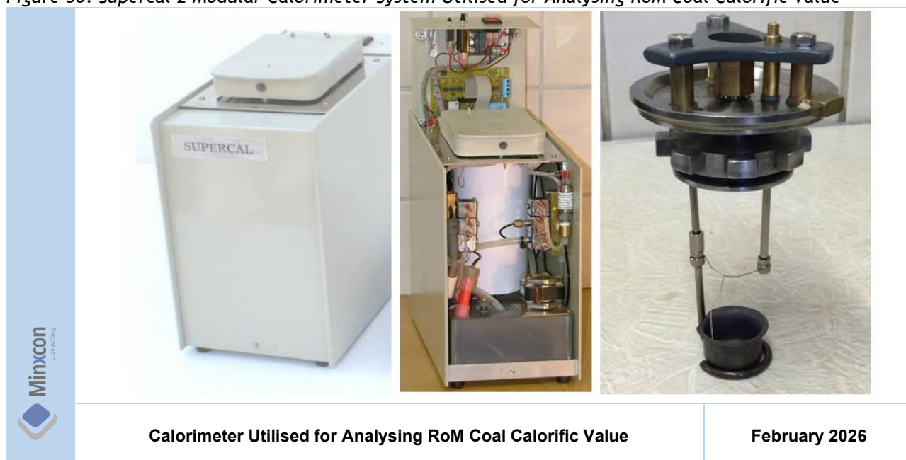
Figure 50: Supercal 2 Modular Calorimeter System Utilised for Analysing RoM Coal Calorific Value
