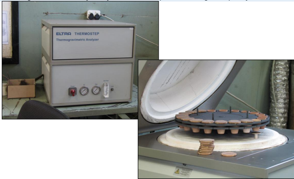
Figure 45: The Thermogravimetric Analyser System Utilised for Measuring LOI of Clay
