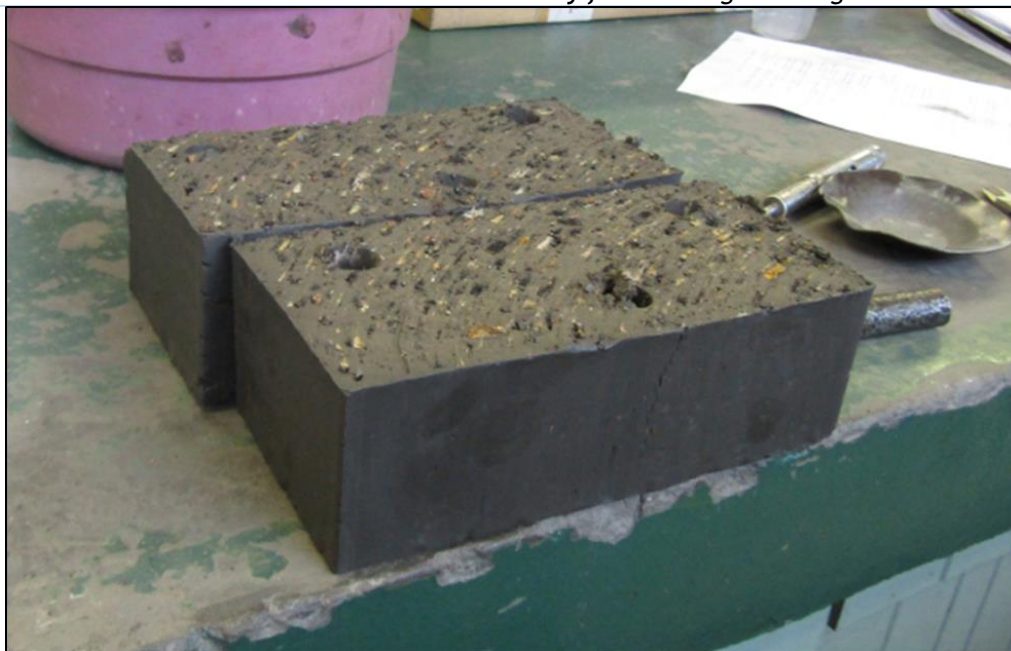
Figure 48: Green Full-sized Bricks Presented to the Laboratory for Shrinkage Testing
